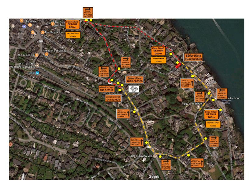
Fig. 3 - Proposed Advance Warning Signage and Diversion Route
